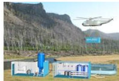
Compact systems are designed and assembled for treatment of a small water quantity from different sources so that they can ensure production of high-quality drinking water.
